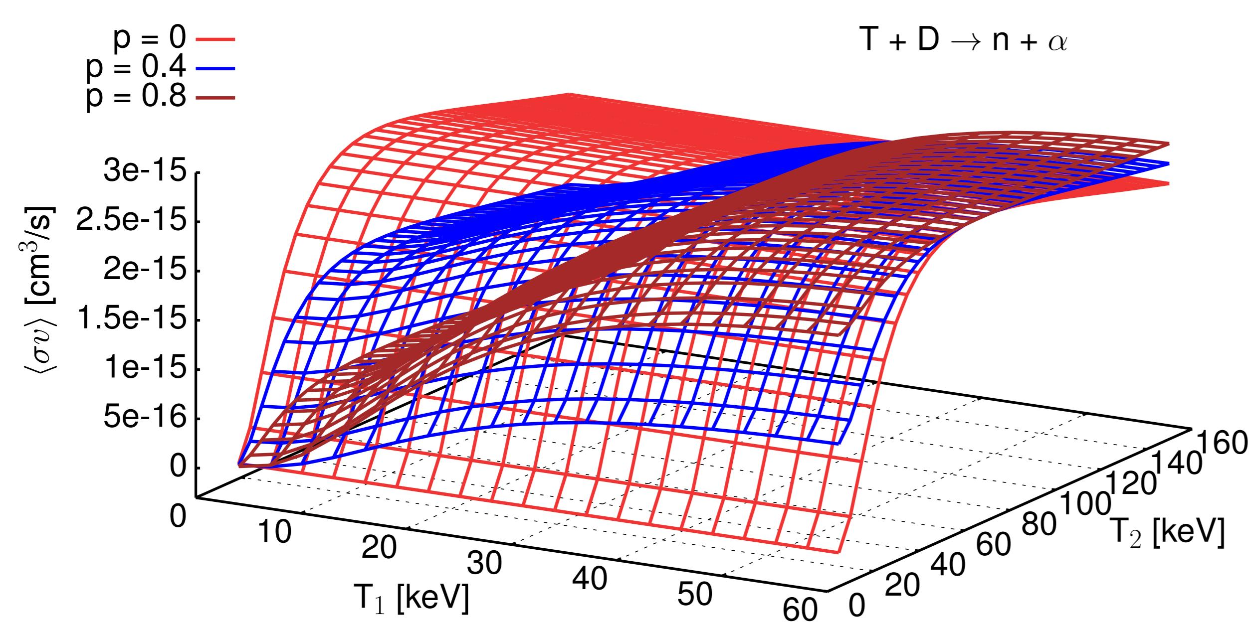
The most effective is to run DT reaction at temperature 64 keV.
