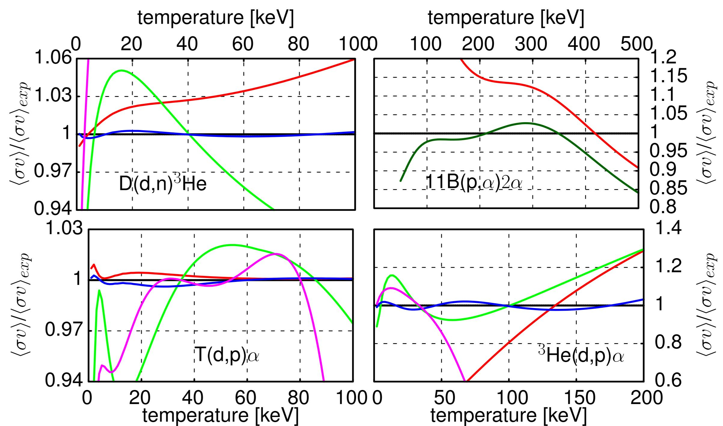
The positions of graphs and colours of lines agree with the figure on the left side. The most precise seems to be to compute reactivity by Bosch&Hale parametrization formula for light nuclei reaction. Nevins&Swain formula satisfies the <sup>11</sup>Bp reactivity data sufficiently.
