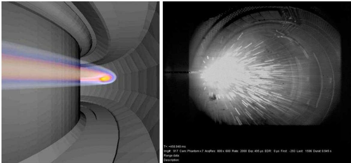
The left figure has been obtained by using synchrotron emission to generate a view of the runaway beam in the DIII-D tokamak in San Diego, USA. The right figure shows the carbon dust generated when runaways hit plasma-facing components in the French tokamak Tore Supra.
