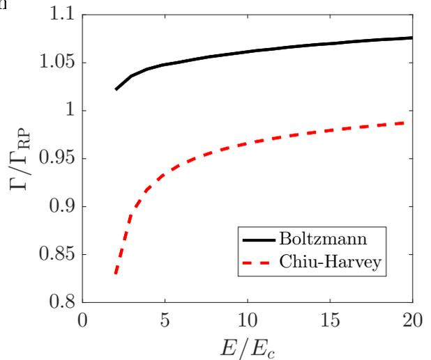
FIG. 4: Avalanche growth rate as function of electric field using different models for the avalanche source rate, normalized to values obtained in the Rosenbluth-Putvinski model.
