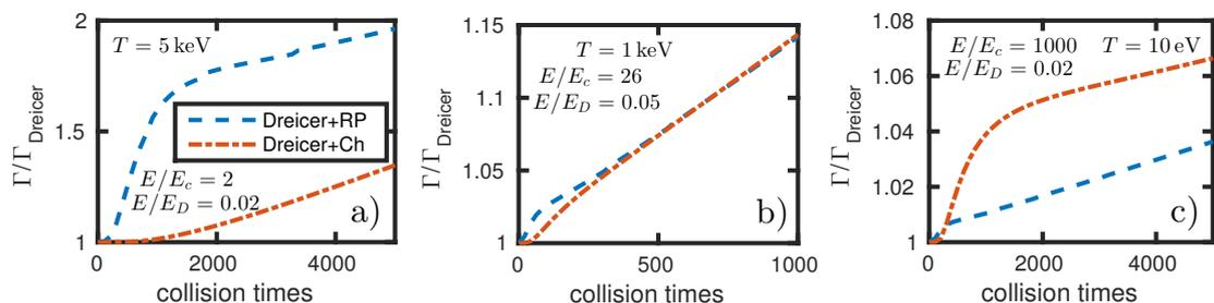
FIG. 3: Runaway growth rates normalized to the Dreicer growth rate for three different scenarios. Blue dashed and red dash-dotted are for the avalanche source terms in Ref. [24] and Ref. [23], respectively. Substantial changes between the two operators can be expected either when the temperature is high and the electric field is low (Ref. [23] over-predicts) or when the temperature is low and the electric field is large (Ref. [23] under-predicts).
