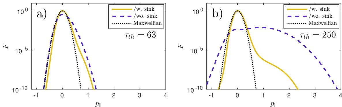
FIG. 2: Cut along the parallel axis of the distribution function after a) 63 and b) 250 thermal collision times in a NORSE run with a constant electric field of  $E = 0.15$  V/m.  $n_e = 5 \cdot 10^{19} \text{ m}^{-3}$ ,  $Z_{\text{eff}} = 1$  and  $B = 0$  T were used, and with the initial temperature  $T_e = 5.11$  keV, the electric field corresponds to  $E/E_D = 0.035$  and  $E/E_c = 3.5$ . The distributions are normalized to their initial maximum value.
