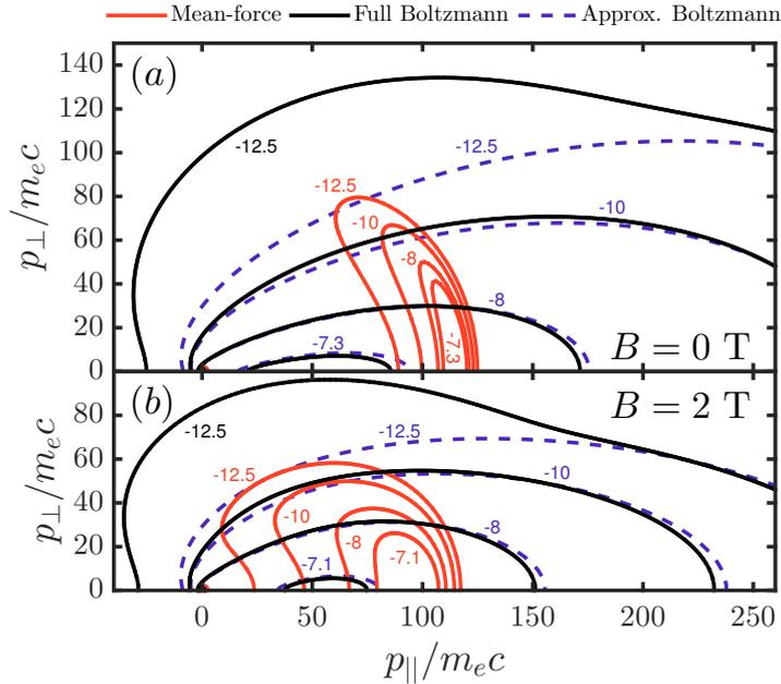
FIG. 1: Steady-state electron 2D distribution functions with (a) no magnetic field and (b)  $B = 2$  T. The other parameters are electric field  $E = 2E_c$ , effective charge  $Z_{\text{eff}} = 10$ , electron density  $n_e = 3 \cdot 10^{21} \text{ m}^{-3}$  and temperature  $T_e = 10 \text{ keV}$ . Contours of  $\log_{10} F$  are shown, where  $F = (2\pi m_e T_e)^{3/2} f_e/n_e$ .
