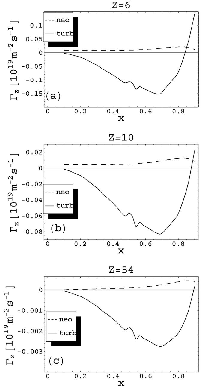
FIG. 5. Neoclassical (dashed) and turbulent (solid) impurity particle transport as a function of normalized radius  $x=r/a$  for impurity charges  $Z=6, 10, 54$ .
