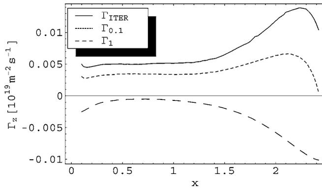
FIG. 2. Neoclassical impurity particle transport for the selected ITER scenario (solid), for a flat density profile with  $n_{0,1}=n_i(0)(1-(r/a)^2)^{0.1}$  (dotted), and for a peaked density profile  $n_1=n_i(0)(1-(r/a)^2)$  (dashed) as functions of radius for impurity charge  $Z=10$ . Note that the neoclassical transport is outward only for flat density profiles.
