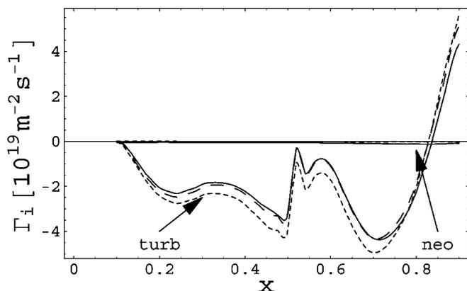
FIG. 7. Main ion turbulent and neoclassical transport as a function of normalized radius  $x=r/a$ , for  $Z=6$  (solid),  $Z=10$  (dashed),  $Z=54$  (dotted). The turbulent transport is inward except for the edge plasma.
