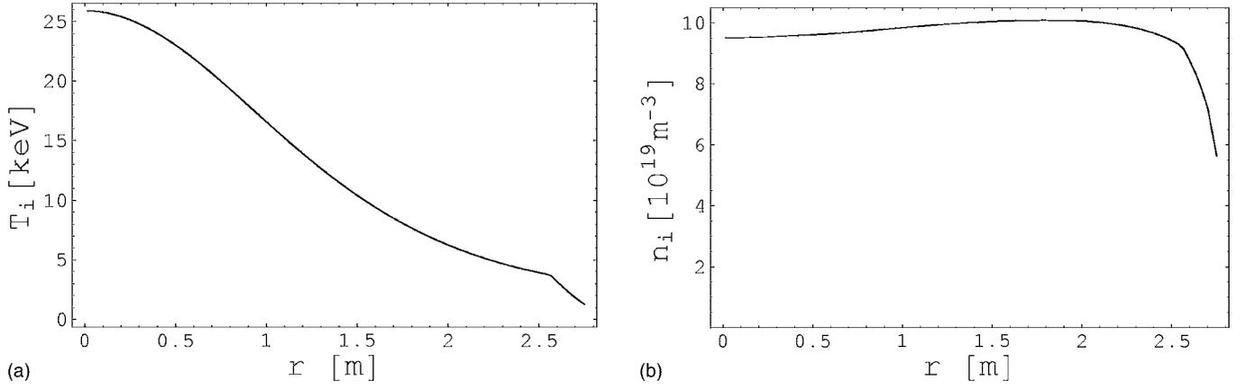
FIG. 1. Radial temperature and density profiles as a function of minor radius in the ITER high- $Q$  scenario.
