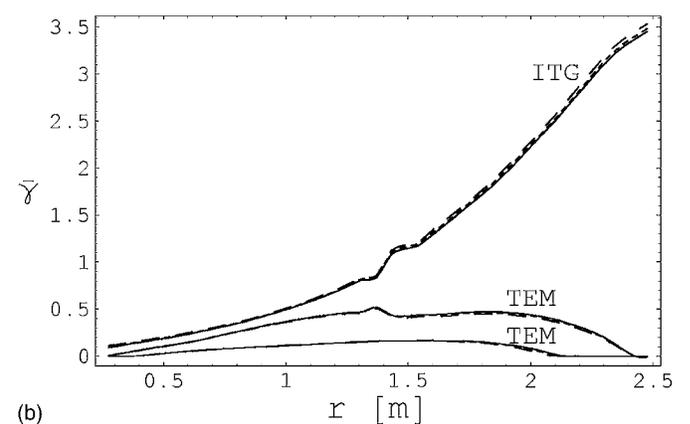
FIG. 4. The real part of the frequency  $\bar{\omega}_r$  and the growth rate  $\bar{\gamma}$  of the unstable ITG mode and the two most unstable TEM modes, normalized to the electron magnetic drift frequency, for  $Z=6$  (solid),  $Z=10$  (dotted),  $Z=54$  (dashed). The curves for different impurity charges overlap, indicating that the frequency and growth rate of the unstable modes are not sensitive to  $Z$ . The ITG mode has negative real frequency and larger growth rate than the TEM modes.
