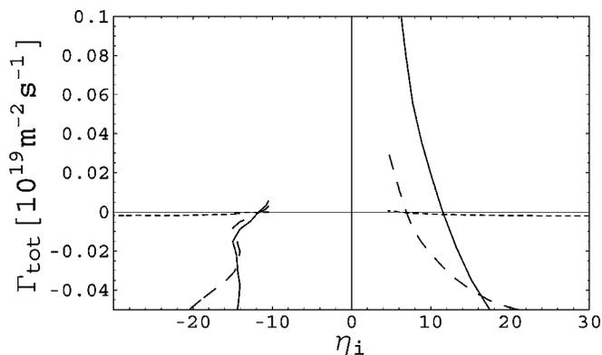
FIG. 6. Total (turbulent + neoclassical) impurity transport as a function of  $\eta_i$ , for  $Z=6$  (solid),  $Z=10$  (dashed),  $Z=54$  (dotted). For large  $Z$ , the impurity transport is always inward, but weak. For low  $Z$ , the impurity transport depends sensitively on  $\eta_i$ .
