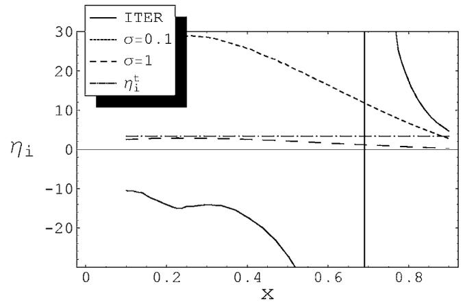
FIG. 3.  $\eta_i$  for the density profiles used in Fig. 2 as functions of  $x=r/a$  together with the threshold for  $\eta_i$ , denoted by  $\eta_i^t$ , for  $Z=10$ . If  $\eta_i > \eta_i^t$  or  $\eta_i < 0$ , the neoclassical impurity transport is outward.
