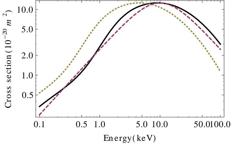
FIG. 1. Cross sections for charge exchange of  $D^+$  with  $N_2$  as a function of projectile energy. Dashed line shows the fit  $\sigma_x^D = (5/2)E_k/(1 + (0.1E_k)^2)10^{-20} \text{ m}^2$  and dotted line shows the cross-section for charge exchange of  $H^+$  with  $N_2$ .
