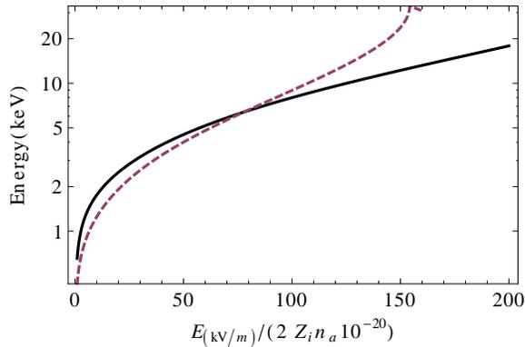
FIG. 3. Ion energy obtained as the solution of  $T_i = Z^2 e E / (2 Z_i n_a \sigma_x)$ . Solid line is for deuterium ions, dashed line is for protons.
