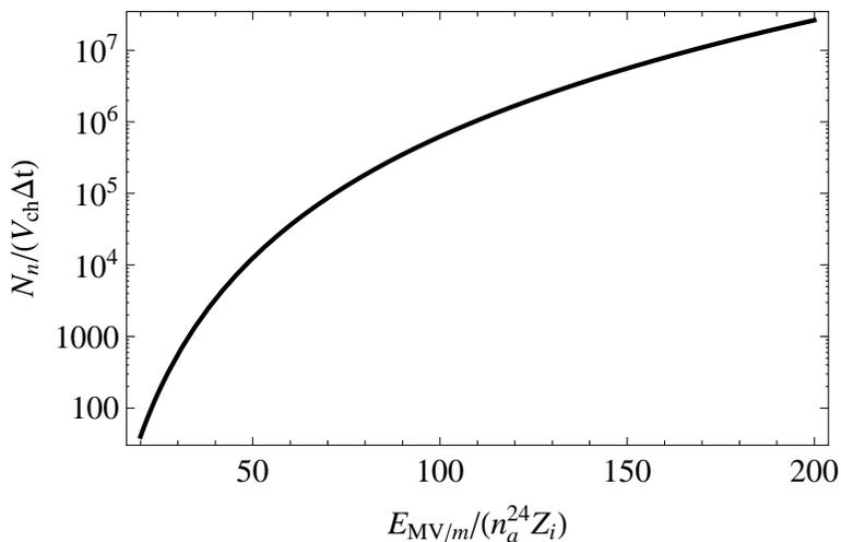
FIG. 4. Number of neutrons as function of  $E/(n_a Z_i)$ , where  $E$  is in  $\text{MV/m}$  and  $n_a$  is in units of  $10^{24} \text{ m}^{-3}$ .
