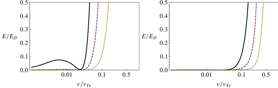
FIG. 2.  $E/E_D$  from Eq. (2) as a function of the deuterium ion speed normalized to the electron thermal speed. (a) The electron density is  $n_e = 10^{21} \text{ m}^{-3}$ . Solid is for mean ionic charge  $Z_i = 0.1$ , dashed is for  $Z_i = 0.01$  and dotted is for  $Z_i = 0.001$ . (b) The mean ionic charge is  $Z_i = 0.001$ . The electron density is  $n_e = 10^{21} \text{ m}^{-3}$  (solid),  $n_e = 10^{22} \text{ m}^{-3}$  (dashed),  $n_e = 10^{23} \text{ m}^{-3}$  (dotted).
