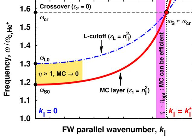
FIG. 3: Normalized IIIH resonance and L-cutoff frequencies as a function of the FW parallel wavenumber.
