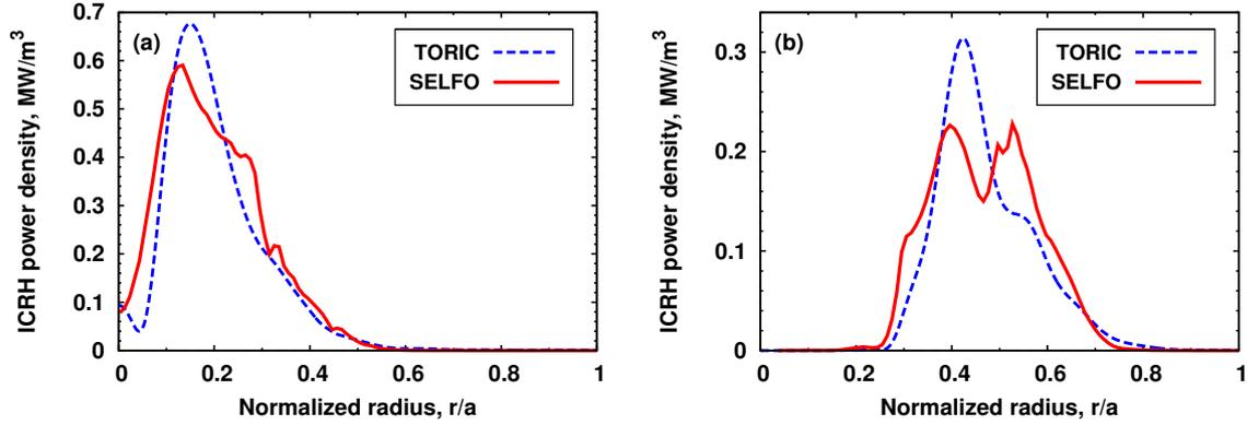
**Figure 5.** Flux surface averaged deposition profiles to hydrogen minority ions calculated with the TORIC (dashed) and the SELFO codes (solid) for  $B_0 = 2.9$  T (a) and  $B_0 = 3.1$  T (b).
