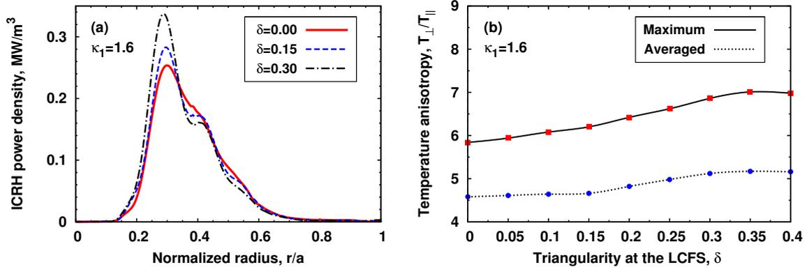
**Figure 3.** Flux surface averaged absorption profiles (a) and minority temperature anisotropy (b) evaluated by the TORIC-SSFPQL for various values of the plasma triangularity. The LCFS ellipticity is  $\kappa_1 = 1.6$ .
