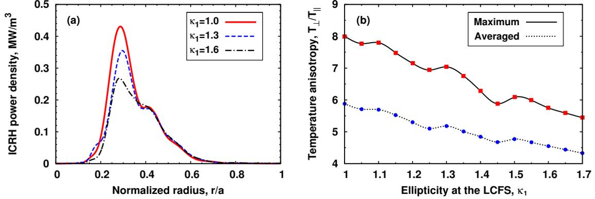
**Figure 1.** Flux surface averaged absorption profiles (a) and minority temperature anisotropy (b) evaluated by the TORIC-SSFPQL for various values of the ellipticity at the LCFS. The input ICRH power is  $P_{\text{ICRH}} = 3.0$  MW.
