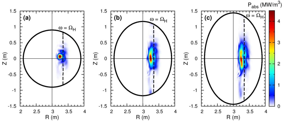
**Figure 2.** Contour plots of the RF power deposition to hydrogen minority ions in the poloidal cross-section from the TORIC simulations for different values of the edge ellipticity: (a)  $\kappa_1 = 1.0$ , (b)  $\kappa_1 = 1.3$ , (c)  $\kappa_1 = 1.6$ .
