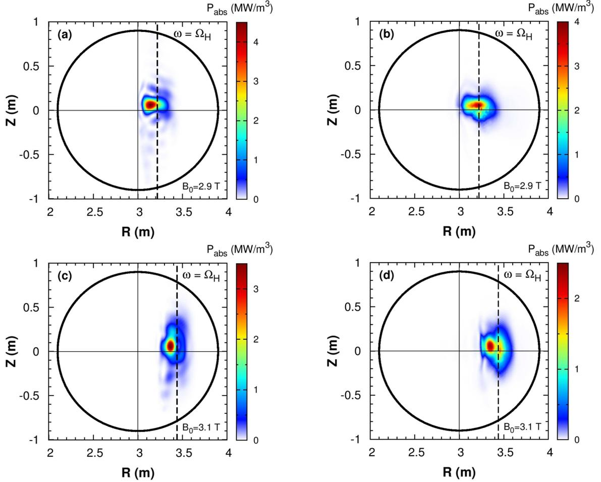
**Figure 4.** Contour plots of the RF power deposition to hydrogen minority ions in the poloidal cross-section calculated with the TORIC (a,c) and the SELFO (b,d) codes for  $B_0 = 2.9$  T and  $B_0 = 3.1$  T.
