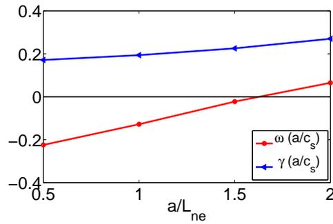
**Figure 10.** Real and imaginary parts of the eigenvalues as function of  $a/L_{ne}$  obtained by GYRO. Red lines (with circle markers) represent the real part, blue lines (triangle markers) correspond to the imaginary part of the eigenvalue. The frequencies are normalized to  $c_s/a$ .
