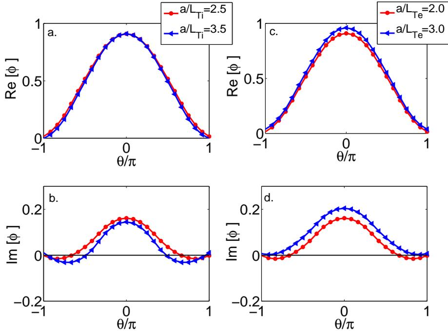
**Figure 6.** Real and imaginary parts of the electrostatic potentials in the cases corresponding to Fig. 5 for different ion- (a,b) and electron (c,d) temperature gradients. (a) and (c) show the real parts and (b) and (d) show the imaginary parts of  $\phi$  (note the different scale). Red lines (circle markers) show the temperature gradient corresponding to the baseline case and blue lines (triangle markers) show the case with the larger temperature gradient.
