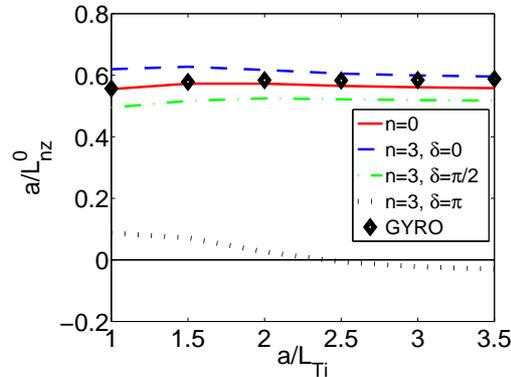
**Figure 13.** Peaking factor for nickel as a function of ion temperature gradient for different values of  $\delta$ , without taking into account parallel compressibility. Solid (red) line represents the case of poloidally symmetric impurity distribution; in figures (a-c) this is compared to GYRO simulations (black diamonds). Out-in asymmetry (dashed, blue) up-down asymmetry (dash-dotted, green), in-out asymmetry (dotted, black).
