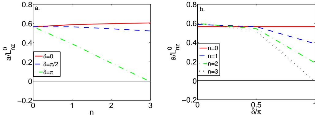
**Figure 12.** Peaking factor for nickel as a function of  $n$  (a) and  $\delta$  (b), without taking into account parallel compressibility. (a): symmetric impurity density (solid, red), up-down asymmetry (dashed, blue), and in-out asymmetry (dash-dotted, green). (b): in-out asymmetry – symmetric impurity density (solid, red),  $n = 1$  (dashed, blue),  $n = 2$  (dash-dotted, green) and  $n = 3$  (dotted, black).
