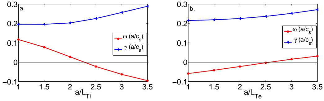
**Figure 5.** Real and imaginary parts of  $\omega = \omega_r + i\gamma$  as function of  $a/L_{Ti}$  (a) and  $a/L_{Te}$  (b) obtained by GYRO for the baseline case. Blue lines (with circle markers) represent the real part, blue lines (triangle markers) correspond to the imaginary part of the eigenvalue. The frequencies are normalized to  $c_s/a$ .
