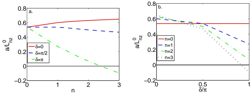
**Figure 4.** Peaking factor for nickel as a function of  $n$  (a) and  $\delta$  (b). (a): symmetric impurity density (solid, red), up-down asymmetry (dashed, blue), and in-out asymmetry (dash-dotted, green). (b): symmetric impurity density (solid, red),  $n = 1$  (dashed, blue),  $n = 2$  (dash-dotted, green), and  $n = 3$  (dotted, black).
