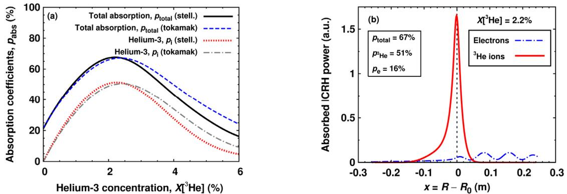
**FIGURE 3.** (a) Single-pass absorption coefficients in  $({}^3He)$ -H plasma vs. the concentration of helium-3 ions evaluated with the baseline and modified versions of the TOMCAT solver. (b) Radial ICRH power deposition profiles for  $X[{}^3He] = 2.2\%$ .
