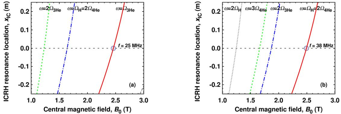
**FIGURE 2.** Locations of the ICRH resonance layers for different ion species vs.  $B_0$  for the lowest,  $f = 25$  MHz (a) and highest,  $f = 38$  MHz (b) frequencies within frequency range available for TEXTOR generators, which will be used in W7-X.
