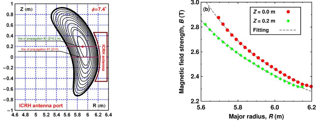
**FIGURE 1.** (a) Port for ICRH antenna in W7-X is reserved at the toroidal angle  $7.4^\circ$  facing the bean-shaped plasma. (b) Radial variation of the magnetic field strength along the lines of wave propagation  $Z = 0.0$  m and  $Z = 0.2$  m.
