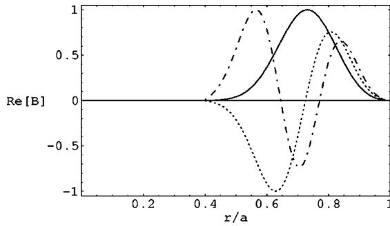
FIG. 2. Radial variation of the real part of the magnetic field  $\hat{B}$  for  $R_0/a = \infty$ , density profile  $n_i(r) = n(0)(1 - (r/a)^2)^{0.5}$  and circular cross section. The eigenfrequencies are  $\omega = 3 \omega_c$  (solid),  $\omega = 3.25 \omega_c$  (dotted), and  $\omega = 3.5 \omega_c$  (dash-dotted).
