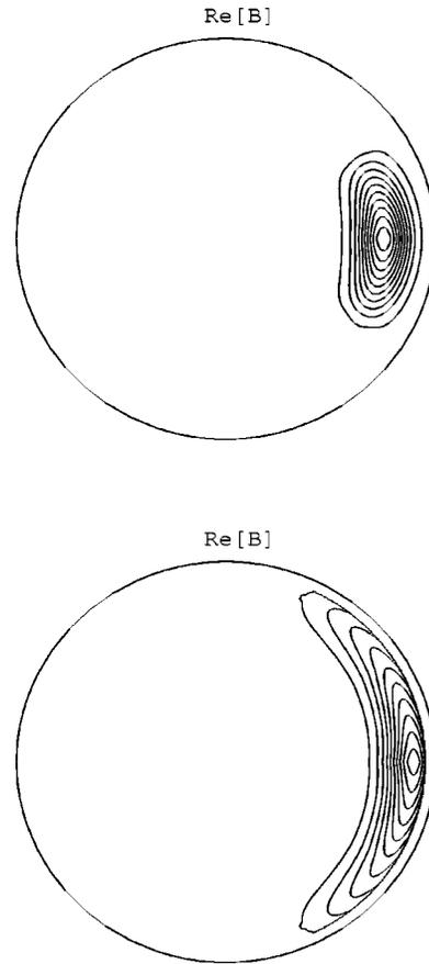
FIG. 3. Poloidal variation of the real part of the magnetic field  $\hat{B}$  for aspect ratio  $R_0/a = 3$ , density profile  $n_i(r) = n(0)(1 - (r/a)^2)^{0.5}$ , circular cross section,  $n = 0$  and (a)  $\omega = 3.1 \omega_{ci}$ ,  $m = -25$ ; (b)  $\omega = 2.4 \omega_{ci}$ ,  $m = 25$ .
