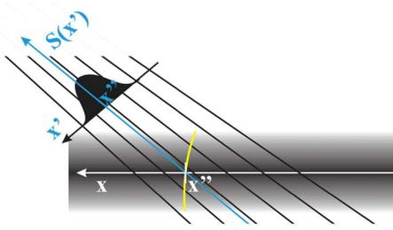
FIG. 1. (Color online) Construction of the transfer function of the observation.  $x$  is the coordinate along the beam axis, which is one-to-one mapped to  $x'$  through the lines of sight crossing the axis. The image  $S(x')$  of a light source being on the flux surface poked by the axis at  $x''$  gives  $T(x', x=x'')$ .
