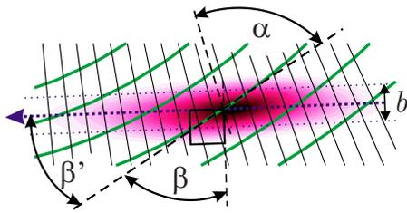
FIG. 10. (Color online) The relevant parameters characterizing the observation geometry.  $b$  is the full width at half maximum of the beam,  $\alpha$  is observation angle,  $\beta'$  is the angle between the beam axis and the flux surfaces, and  $\beta = \pi/2 - \beta'$ . Thick dotted line: beam axis; thick solid curves: flux surfaces; thin solid lines: lines of sight.
