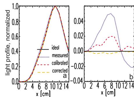
FIG. 9. (Color online) Na-BES, TEXTOR tokamak; (a) light profiles and (b) differences from the ideal light profile.
